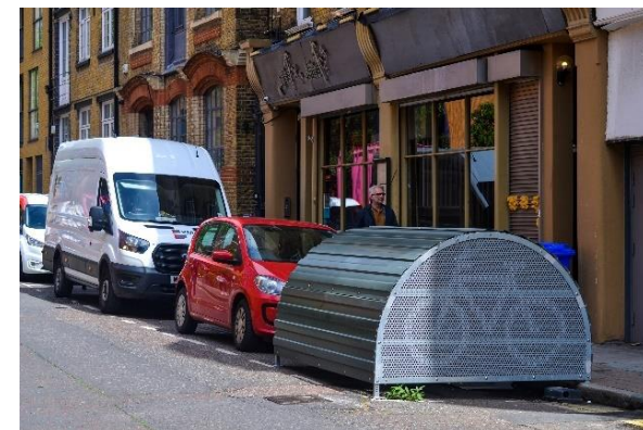
Image 9-7: Bike hangar on space previously used for on-street parking. Hangars provide safe, secure, and sheltered parking for long-stay trips, such as residents of private development or commuters working in old town centre buildings with no space for bike parking. Source: DBFL.
